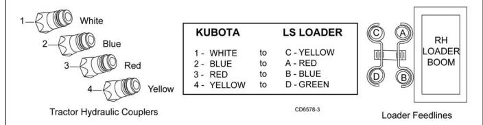
Figure 7. Loader Supply Hose Connections
